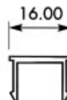
Section No. 5706 Pocket infill 0.122 kg/m, per 75
